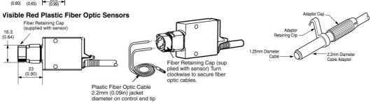
Special Glass Fiber Optic cables are also available with 2.2 mm (0.09 in) diameter control end tips. Note: Cat. No. 61-6731 adaptors are required for smaller fiber optic cables with jacket diameters of 1.25 mm (0.05 in).
