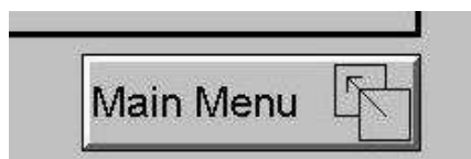
Figure 10.3- Screen Jump Object (configured for a specific screen)
