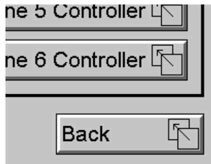
Figure 10.4 - Screen Jump Object (configured to return to previous screen)
