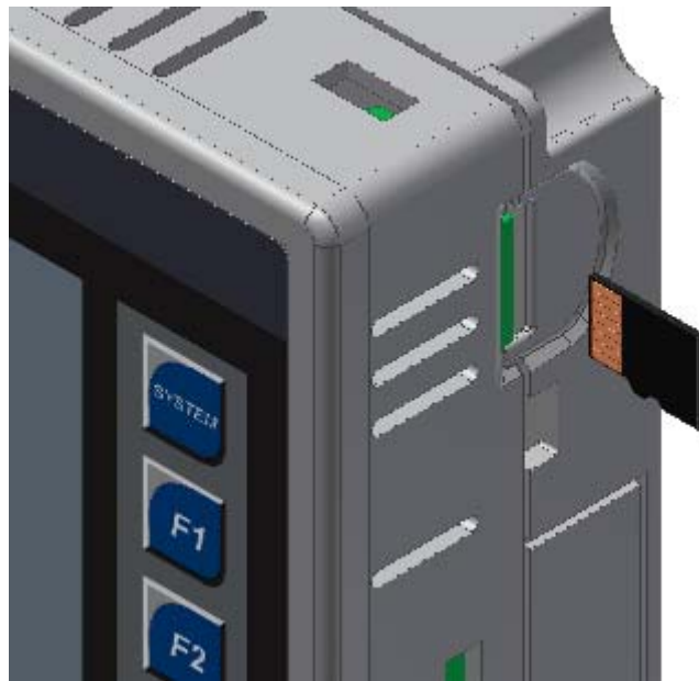
Figure 9.2 – Installing Removable Memory Card
