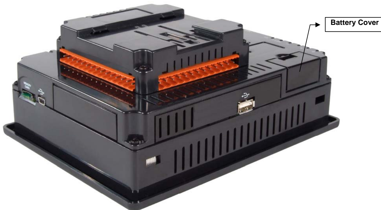
Figure 17.1 – Back Cover - Replacing the back-up battery
