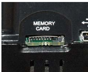
Figure 9.1 – Removable Micro SD Memory Card Slot
