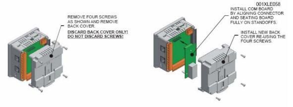
Figure 1 - Removing Back Cover of the XLE
