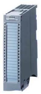
SIMATIC S7-1500, ANALOG OUTPUT MODULE AQ 8 X U/I HS 16 BITS OF RESOLUTION, ACCURACY 0.3 %, 8CHANNELS IN GROUPS OF 8, DIAGNOSIS, SUBSTITUTE VALUE 8 CHANNELS IN 0.125 MS INCL. INFEED ELEMENT, OVERSAMPLING SHIELD CLAMP AND SHIELD TERMINAL
