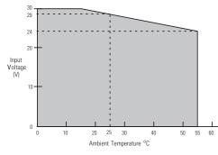
The area within the curve represents the safe operating range for the module under various conditions of user supplied 24V DC supply voltages and ambient temperatures. This includes all possible mounting positions, including inverted horizontal.
