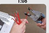
The assembler using the traditional method has measured and cut about 10 of the 18 wires needed for the same job. And there are numerous steps remaining.
