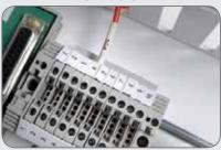
Wiring each terminal block one at a time.
