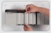
Assembler removes pre-wired 1492 cable from the box and connects the PLC end of the cable to the PLC.
