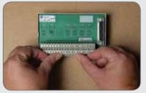
The assembler removes the Bulletin 1492 Interface Module (IFM) from its box and applies the supplied preprinted labels to mark the terminals.
