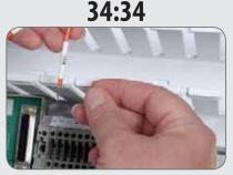
Assembler begins tagging each wire before connecting it to the terminal blocks.
