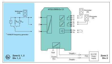
Figure 5.1 Proof test set-up for KF\*\*-DWB-(Ex)1.D
