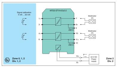
Figure 4.3 Proof test set-up for KFD2-STV4-(Ex)\*-1 and KFD2-STV4-(Ex)\*-2
