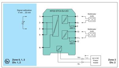
Figure 4.4 Proof test set-up for KFD2-CR4-(Ex)1.2O and KFD2-STC4-(Ex)1.2O Usage in Zone 0, 1, 2/Div. 1, 2 only for Ex versions
