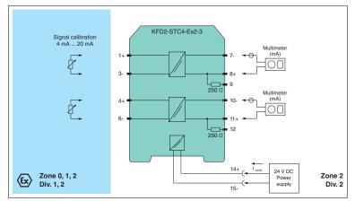
Figure 4.2 Proof test set-up for KFD2-STC4-(Ex)\*-3 and KFD2-STC4-(Ex)\*-Y\*
