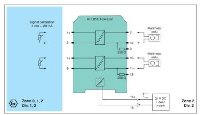
Figure 4.1 Proof test set-up for KFD2-CR4-(Ex)\* and KFD2-STC4-(Ex)\*
