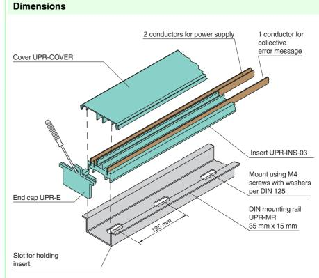
Universal Power Rail with end caps and cover, 3 conductors
